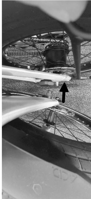
Fig. 7: Close Klickfix Quadlock Adapter
