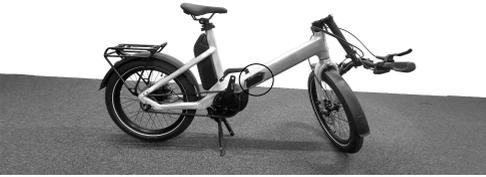
Fig. 4: Unlock folding mechanism
