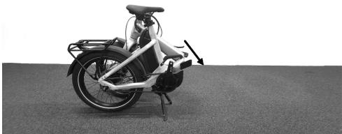
Fig. 11: Swing front frame (open)
