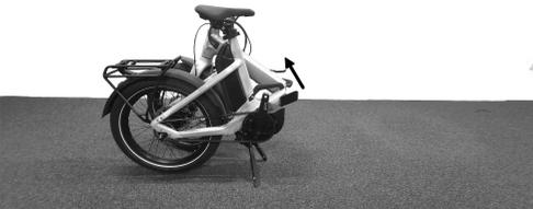
Fig. 6: Swing front frame part (close)
