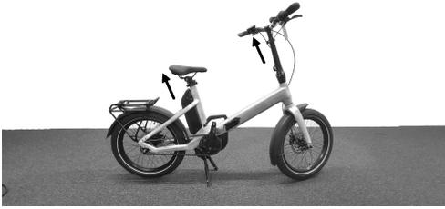
Fig. 15: Adjust stem and saddle height
