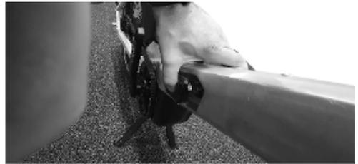
Fig. 13: Lock the folding mechanism by engaging the lever in the ball head
